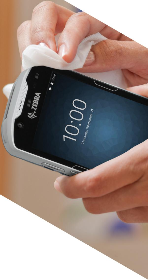
Abrasion presents itself on transparent surfaces as scuff marks, and can make reading a mobile computer screen very difficult for the user or barcode reading nearly impossible for a scan engine. The effects of abrasion on transparent surfaces, such as scanner windows and touch panels, are not reversible by simple means and usually require sending the mobile computer for repair to regain display or scanning functionality.
